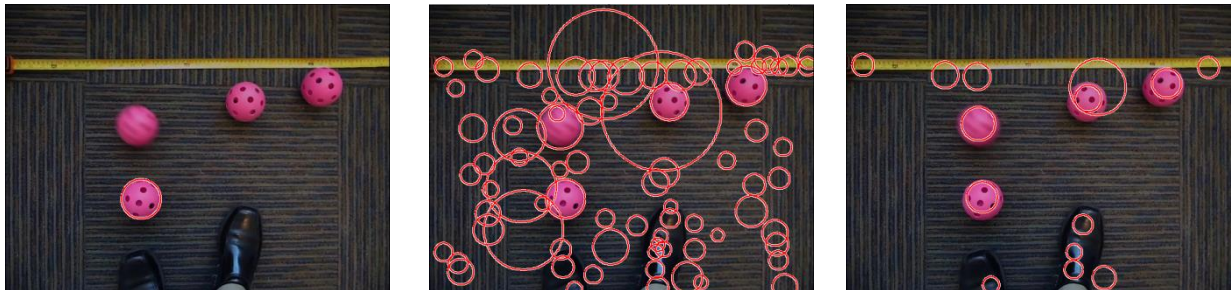
Figure 1: Detected circles for various values of Sensitivity and EdgeThreshold properties including default (left), too high sensitivity (center), too low edge threshold (right) and
